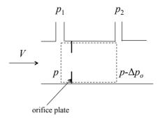
An orifice plate is simply a plate with a hole in it, mounted in a pipe as shown. A force balance follows in a very similar manner to that used in Appendix A, where instead of a shear force at the we have in general viscous losses. Here we connect the non-dimensional pressure loss via dimensional analysis, which is also expected to be a function of the Reynolds number.
